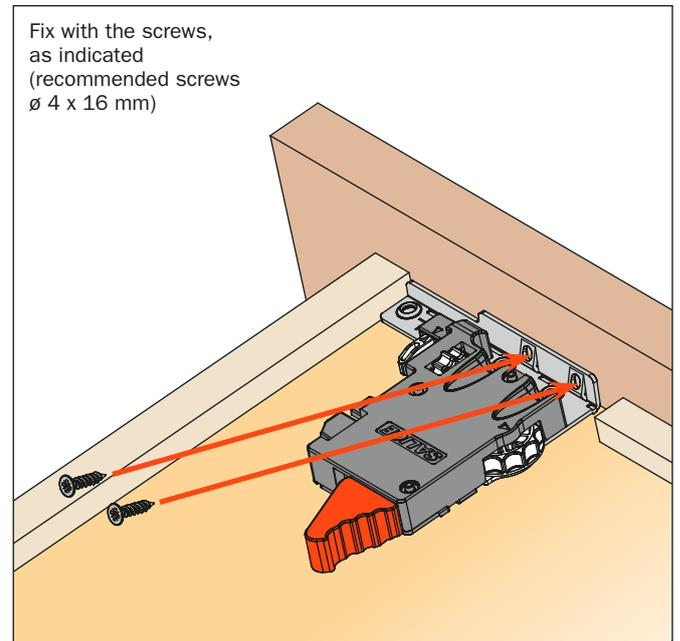
It is recommended to pre-drill the bottom or the frontal using the **SGD704UGXA drilling template**, see page 35.
