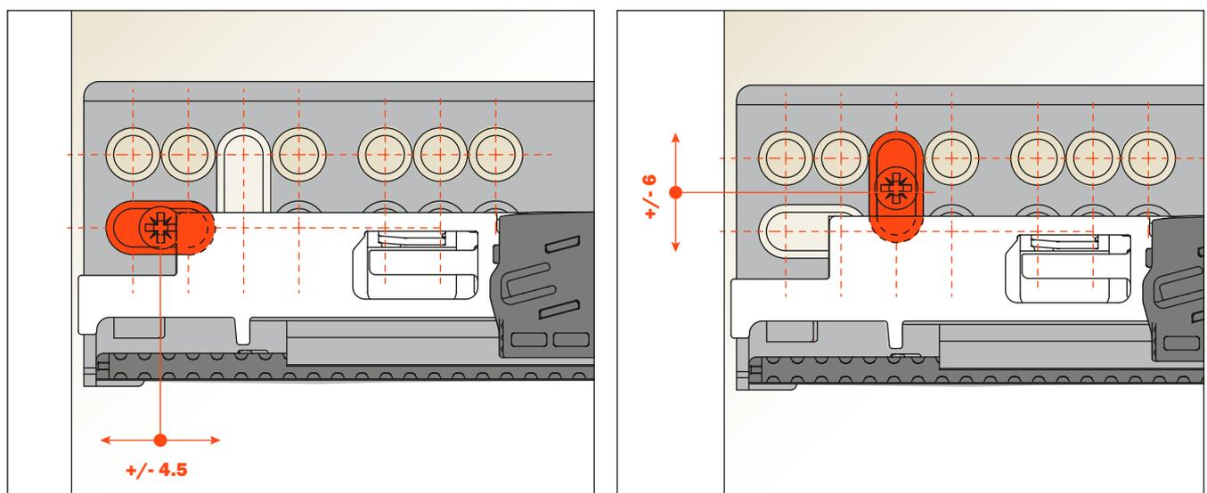
**Drilling positions for runner on cabinet side**
