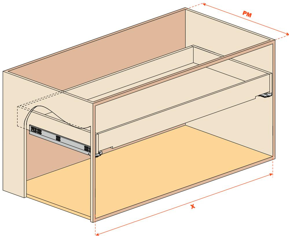
The internal width of the drawer is 42 mm less than the internal width of the cabinet
