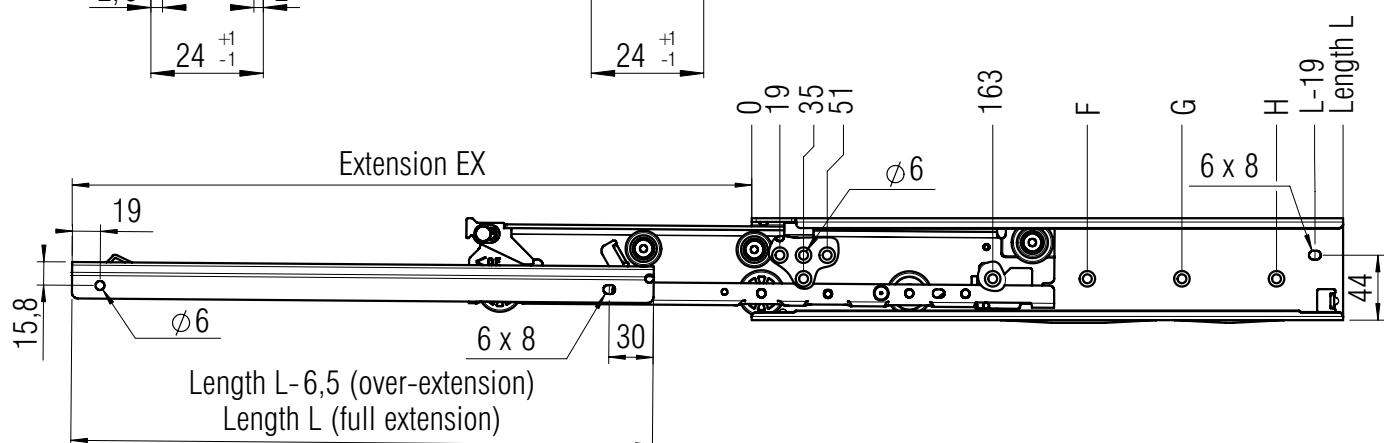
screw holes for 4,5 mm spax screws
